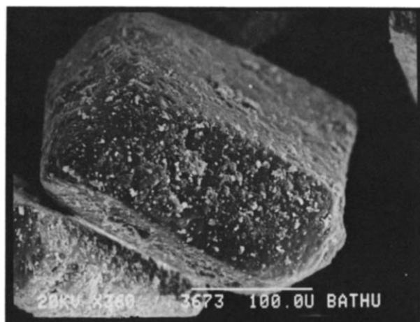
Fig. 5. Scanning electron photomicrograph of a single coarse sucrose carrier particle with a uniform coating of finer adherent triamterene particles.
